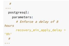
Monitor and adjust the delay as needed based on your recovery time objectives and the potential impact of unintended primary database operations.
