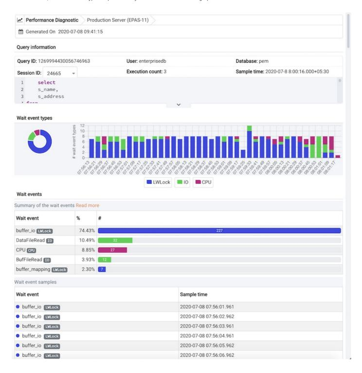
The Wait events section has a table displaying all the wait events that occurred during the query execution. It displays data in decreasing order by number of wait events. The second table displays the wait event with sample times that occurred over the period of the whole query execution. It allows you to analyze the wait events during the query execution over the period of time. Also, it shows the actual samples collected by the EDB Wait States extension for that query ID and session ID.
